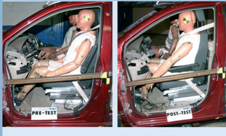
Crash test of a Turny Orbit in a Toyota Sienna.
