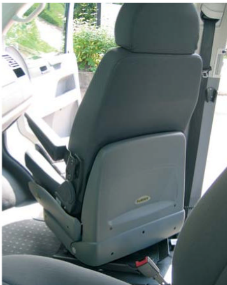
Turny HD fitted with the BEV-seat (an optional extra).
