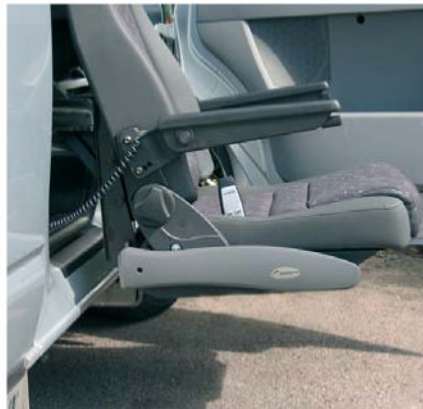
Turny HD fitted with the BEV-seat (an optional extra).
