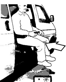
4. When the user is seated press the hand control button for driving up and in. If the movement needs to be interrupted, just release the control button. Mind the head when entering through the door way! Keep the control button pressed down until final position is reached and the green diode is shining.
