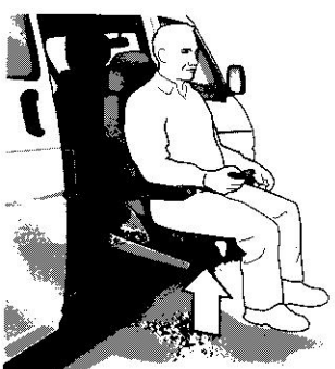
4. When the user is seated press the hand control button for driving up and in. If the movement needs to be interrupted, just release the control button. Mind the head when entering through the door way! Keep the control button pressed down until final position is reached and the green diode is shining.
