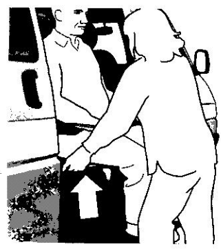
5. Lift the release lever for rotation and rotate the seat inside the vehicle until the Turny locks it in final position.
