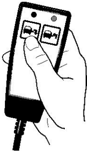
3. Use the control pendant and drive down the seat to a suitable level.
