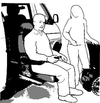
4. When the user is seated press the hand control button for driving up and in. If the movement needs to be interrupted, just release the control button. Mind the head when entering through the door way! Keep the control button pressed down until final position is reached and the green diode is shining.
