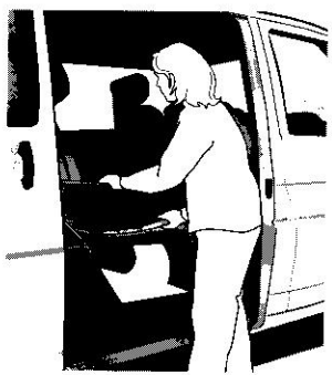
2. Hold on to the seat and rotate it (do not pull it by the release lever). Rotate the seat until maximal outer position.
